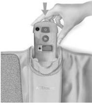
Slide the control unit into its housing on the Compression Sleeve until a click is felt and heard; the control unit is then secured correctly within the sleeve.
